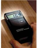
The mini-Scanners are used for measuring the moisture level in finished wood products or other building materials where it is not desirable to leave pin marks on the finished product. It indicates wet and dry moisture levels. This economically priced meter offers state-of-the-art electronics with 8 settings (32 Settings for SD model) to correct for different species. Large easy to read LCD display offers 0.1% resolution.
